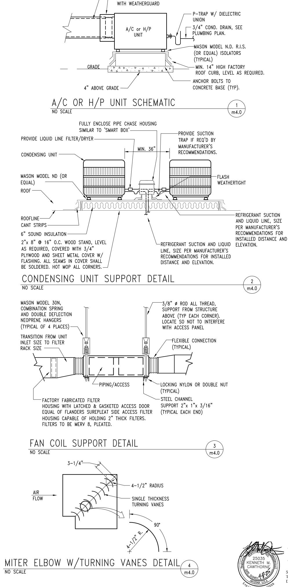
PROVIDE MIN. 2" THICK LINER FOR ALL EXTERIOR SUPPLY AND RETURN DUCT.
