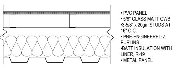
MP EXTERIOR METAL PANEL THICKNESS: 1'-3"
